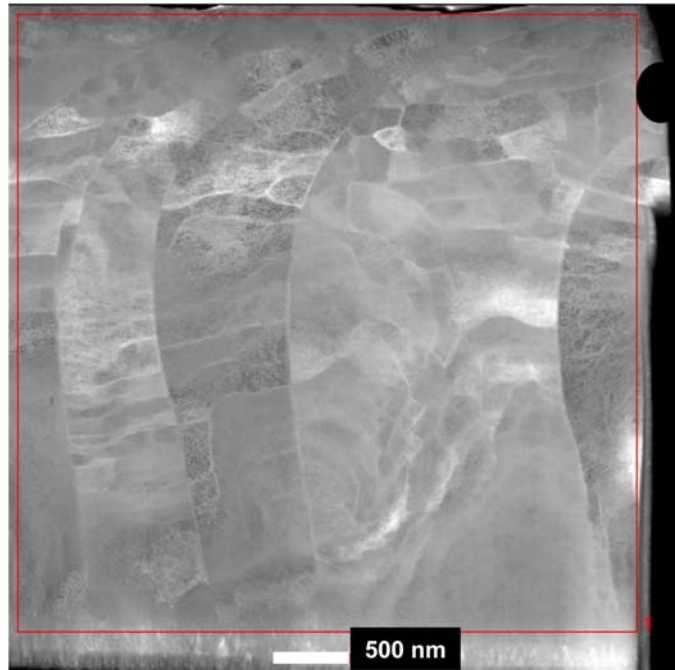
Fig. 13. STEM image of a 4 \times 4 \mu\text{m} region of the TEM thin section from the center of unzoned particle NWA A2H along the direction of the EPMA trace shown in Fig. 1c. The kamacite grains are twisted and plastically deformed. The box identifies the region from which the X-ray scan was obtained.
