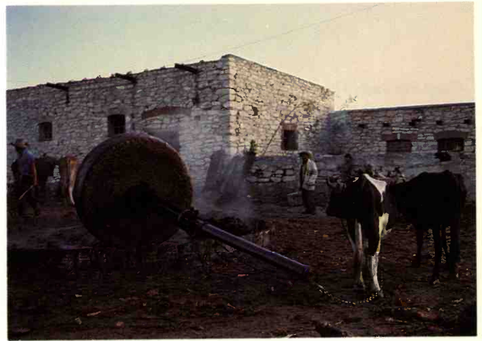
Figure 8. Bovine power has traditionally been harnessed to power the stone mezcal mill. Sometimes nowadays a tractor will be hooked to the stone wheel instead.
