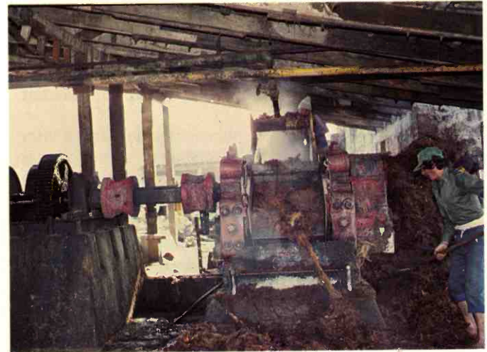
Figure 9. Some mezcal factories now use electric presses in place of the traditional stone mill. The bagazo (fiber) is washed three times.
