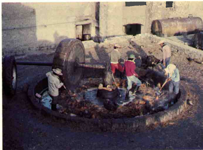
Figure 7. The cooked mezcal is hacked into pieces with axes and crushed with a large stone wheel. Those in charge of this milling process are termed molineros.
