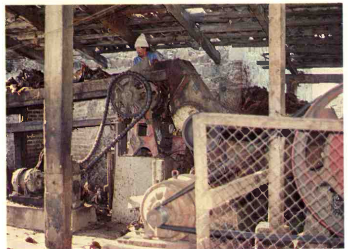
Figure 10. This electric press consists of a large conveyor belt, a shredder, a small conveyor belt, and two sets of press rollers.
