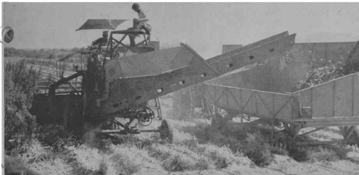
Figure 2. Rear view of combine elevating onion seed stalks into the wagon that is pulled along beside the combine.
