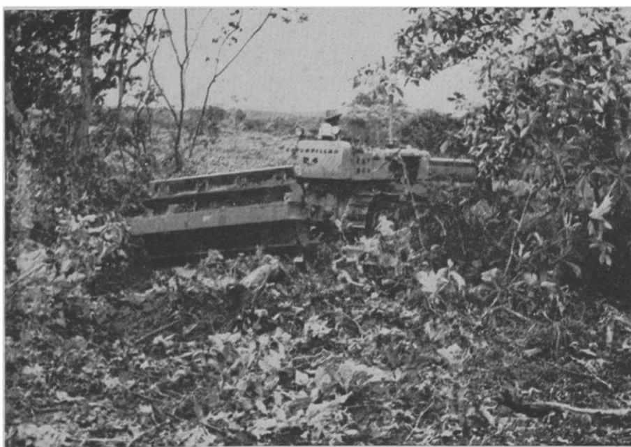
Figure 1. Wet season clearing of a dense stand of brush with the rolling cutter. The cutter was filled with sand and water to increase its weight and usually two passes were made. The debris was burned during the dry season. This brush stand was at least 30 years old.
