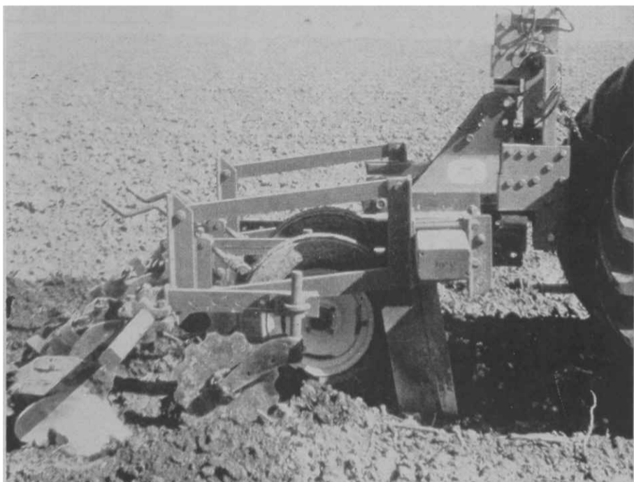
Chisel bed equipment as installed on the tractor is shown above. The arch at hitch point was used to make the draft measurements.
