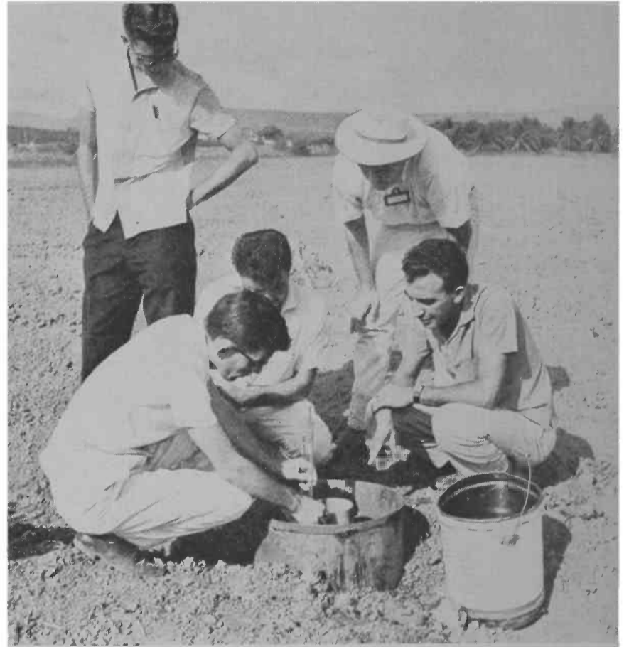
INFILTRATION test, using cylinder infiltrometer.
