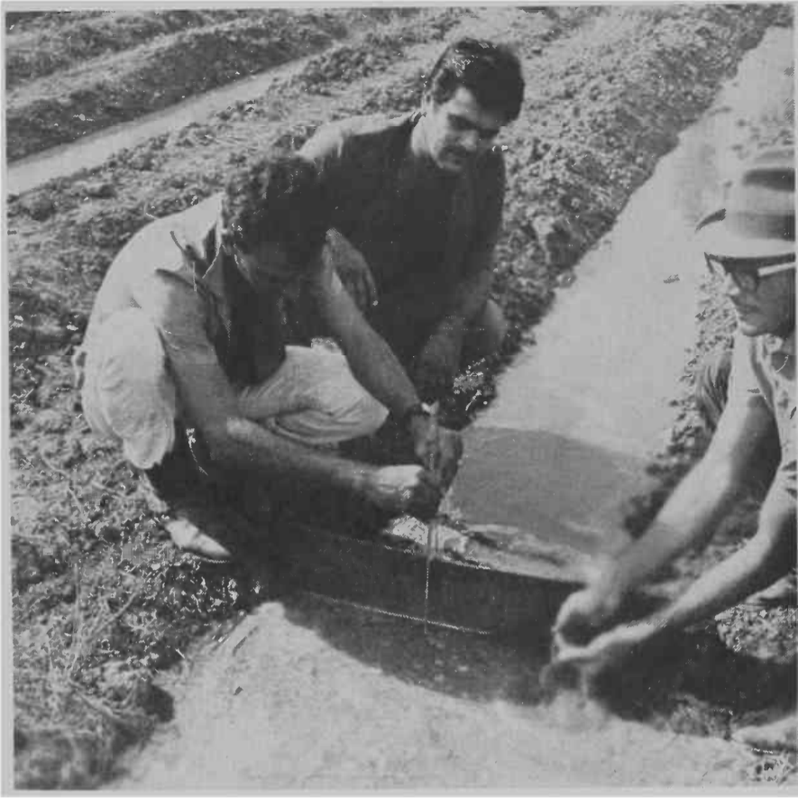
MEASUREMENT of furrow flow with orifice plate.
